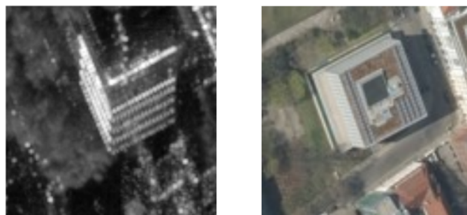
Figure 2.3: Example of co-registered optical and SAR images from the SARptical dataset [23]; large differences in the image geometries become apparent
